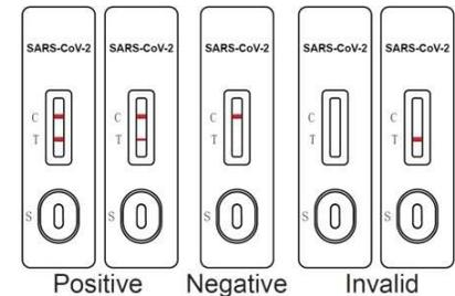
Positive (+): Presence of two red lines, test line (T) and control line (C), indicates SARS-CoV-2 nucleocapsid protein antigens present in samples.
